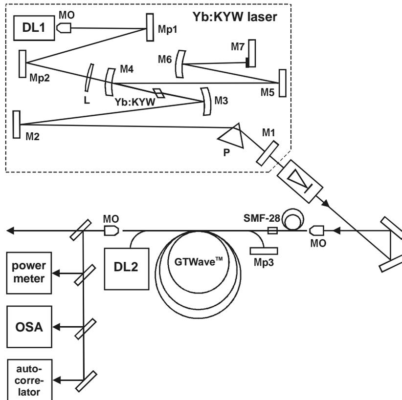
Fig. 1. Schematic experimental setup: DL1/2 – pump diode laser,  $M_{p1/3}$ - reflecting mirrors for pump radiation, M1-M7 - mirrors of Yb:KYW laser, L – lens, P – prism, FI - Faraday isolator, MO - microscope objective.
