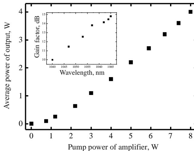
Fig. 6. Experimental results of measurement of average output power versus pump power of amplifier.
