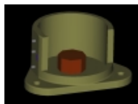
Cut-away view illustrating core sensor component: a Cs vapor cell. Not shown: control electronics.
